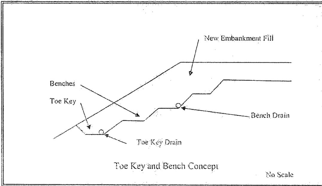
The width of the toe key should be at least one-fourth (1/4) of the height of the fill. The elevation difference between each bench, width, and geometry of each bench is not critical, but generally the elevation difference between each lift should not exceed about three (3) to four (4) feet. The benches should be of sufficient width to allow for placement of horizontal lifts of fill material, therefore the size of the compaction equipment used will influence the bench widths.
