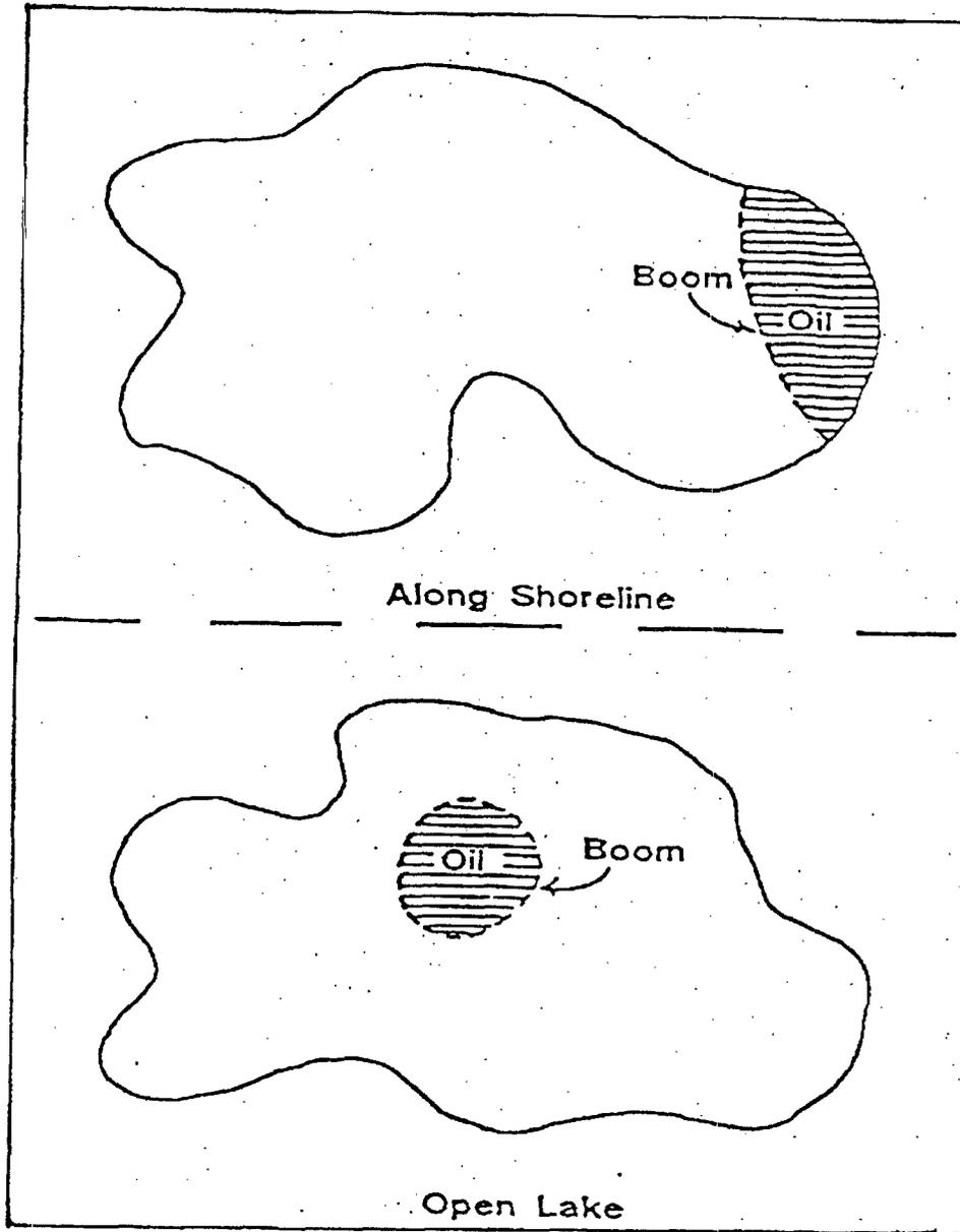
Figure C-1 Boom Deployment in Lakes
