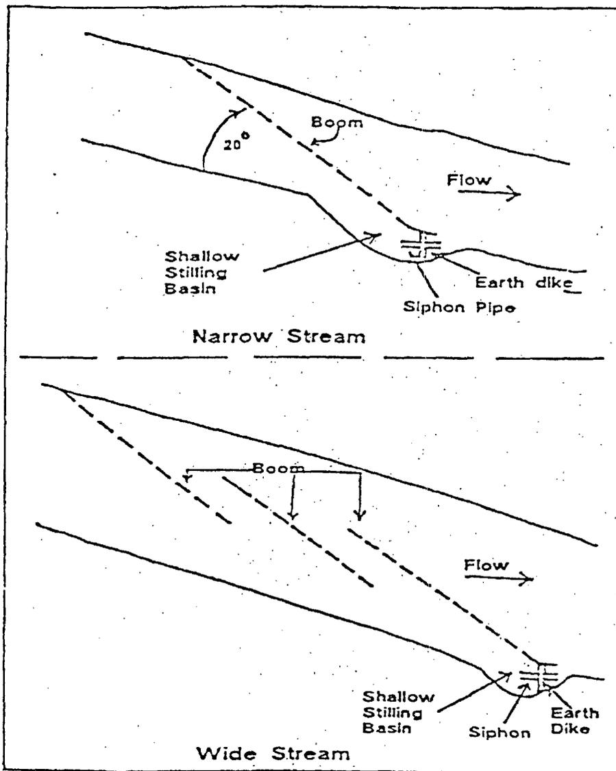
Figure C-3 Boom Deployment in Fast-Flowing Stream
