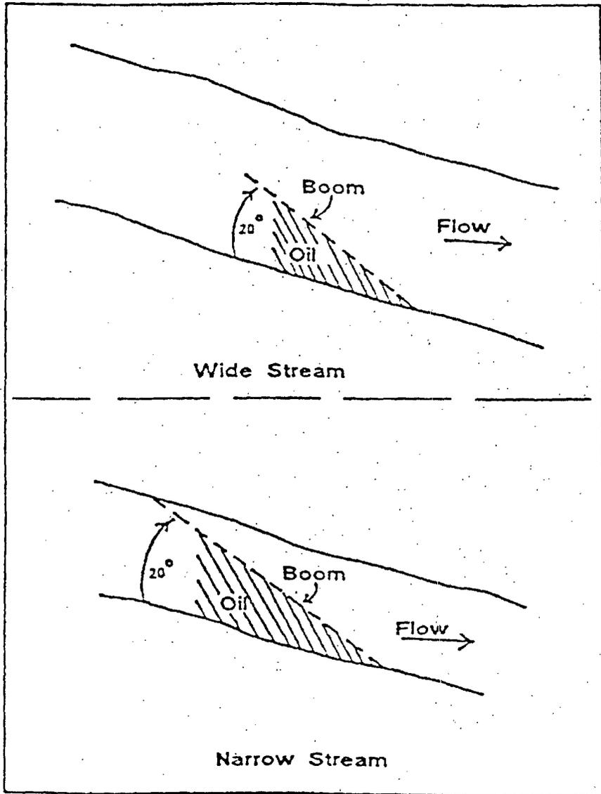
Figure C-2 Boom Deployment in Fast-Flowing Stream
