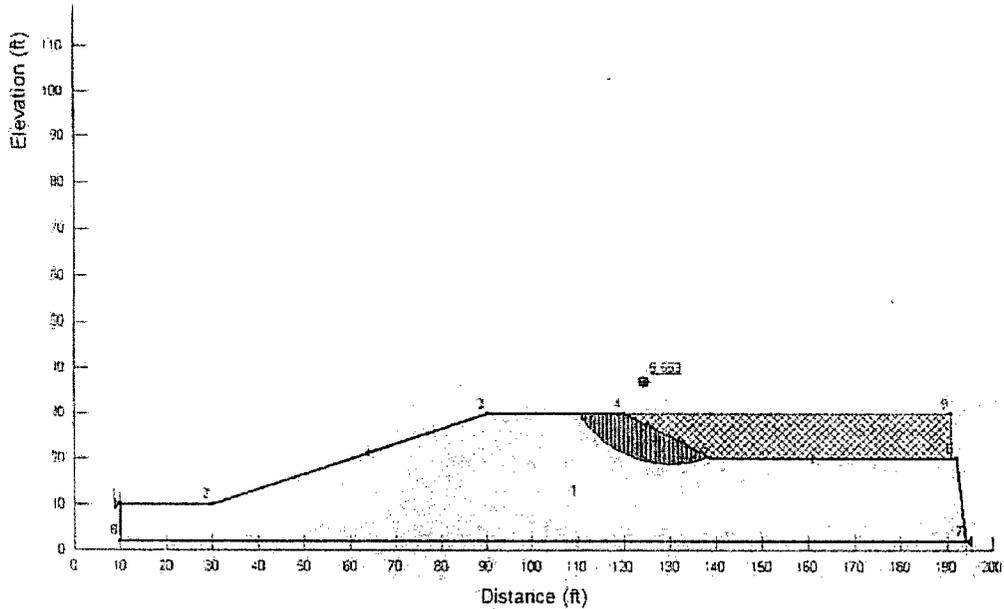
As shown, the theoretical factor of safety of the exterior slope decreases slightly to approximately 2.25 while the theoretical factor of safety of the interior slopes increases substantially to approximately 5.55. The decrease in stability of the exterior slopes and increase in stability of the interior slopes is due to the fluid pressures exerted on the dike by the water. The stability of the geometry shown above may be considered as stable for the proposed lined ponds.
