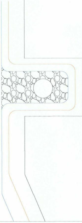
Anchor Trench, located 1' from edge of pond, trench is 1 ft wide X 1' deep
