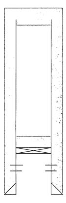
Cut & pulled 2,020' of 5 ½" casing Set 30 sx. cement stub plug 2,000'-2,100'
