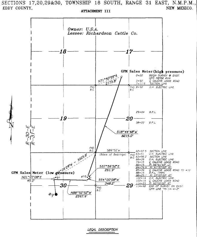
A STRIP OF LAND 50.0 FEET WIDE, LOCATED IN SECTIONS 17,20,29&30 TOWNSHIP 18 SOUTH, RANGE 31 EAST, N.M.P.M., EDDY COUNTY, NEW MEXICO AND BEING 25.0 FEET LEFT AND RIGHT OF THE ABOVE PLATTED CENTERLINE SURVEY.
