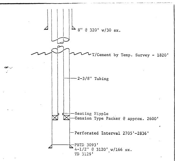
Water will be injected into Oolitic zone of San Andres thru perforated interval 2705-2836' below a tension type packer. The tubing-casing annulus will be loaded with corrosion inhibited fluid.
