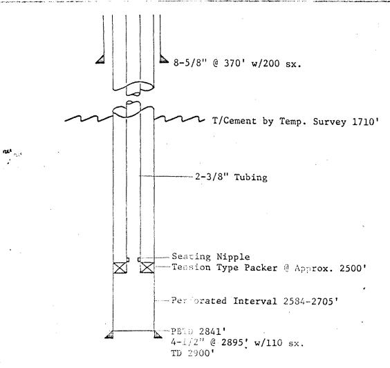
Water will be injected into Oolitic Zone of San Andres thru perforated interval 2584-2705' below a tension type packer. The tubing-casing annulus will be loaded with corrosion inhibited fluid.
