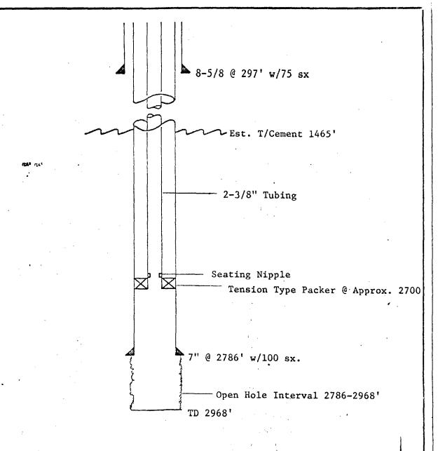
Water will be injected into Oolitic Zone or San Andres in Open Hole 2786-2968'. Below a tension type packer. The tubing-casing annulus will be loaded with corrosion-inhibited fluid.
