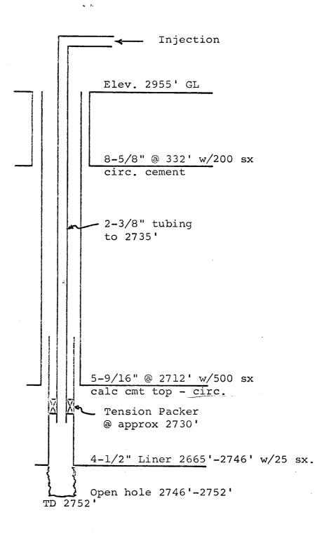
DIAGRAMATIC SKETCH PROPOSED INJECTION WELL 13-2 MALAGA UNIT NW/4 SW/4 Sec. 7-24S-29E Eddy County, New Mexico
