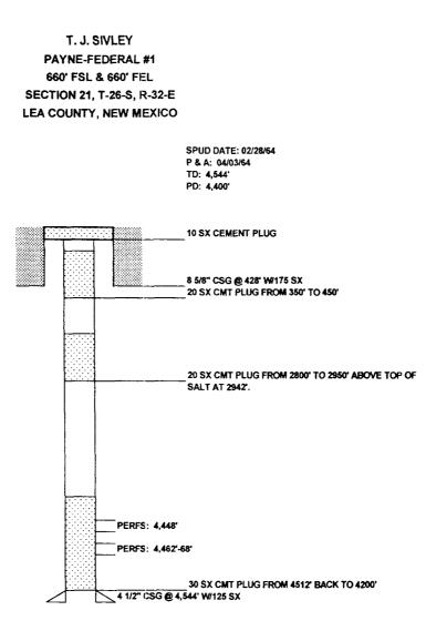
On April 3, 1964 a 30 sack cement plug was spotted from a total depth of 4512' back to 4200', cementing off perforations in 4–1/2" casing located at 4448' and from 4462-68', 4–1/2" casing was then shot off at 3890' for recovery.
