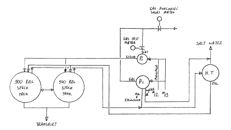
P, - TWO PHASE TEST SEPARATOR P2- THREE PHASE PRODUCTION SEPARATOR H.T. - HEATER TREATER
