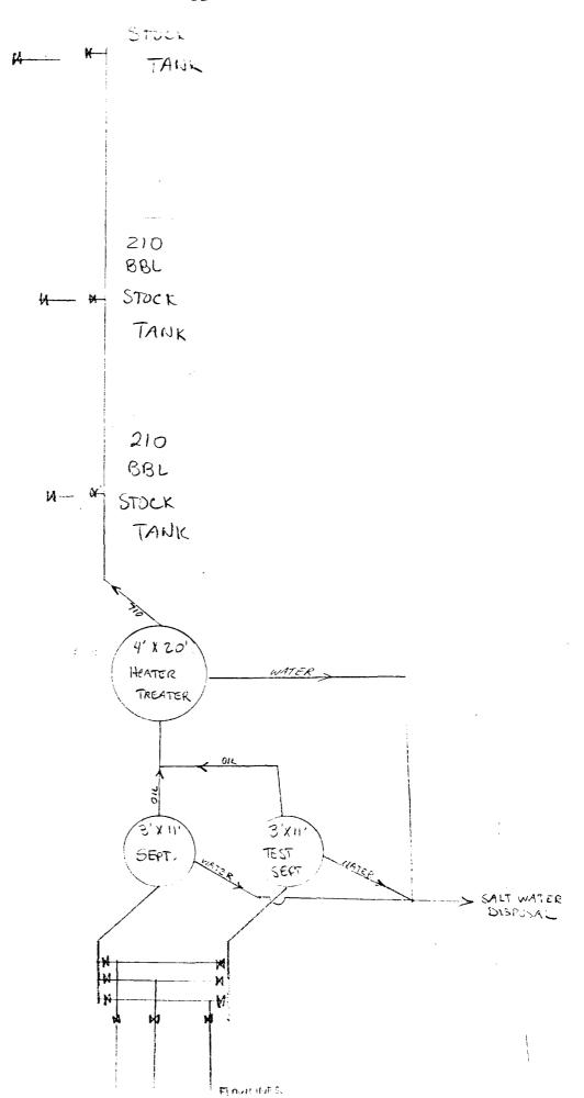
GULF OIL CORPORATION SCHEMATIC TANK BATTERY DIAGRAM R. R. Bell (NCT-E) Lease
