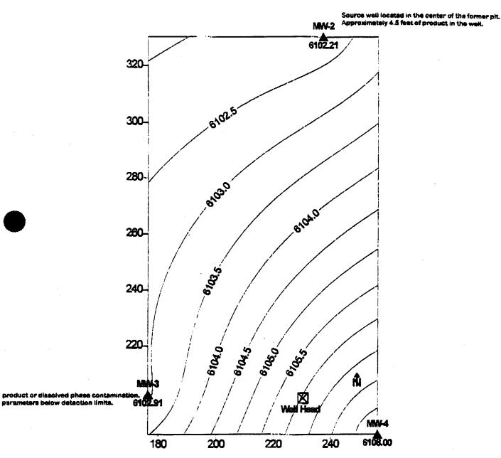
Well is located near product tank batteries and separators. Discolved phase contamination (banzane=811 ppb)
