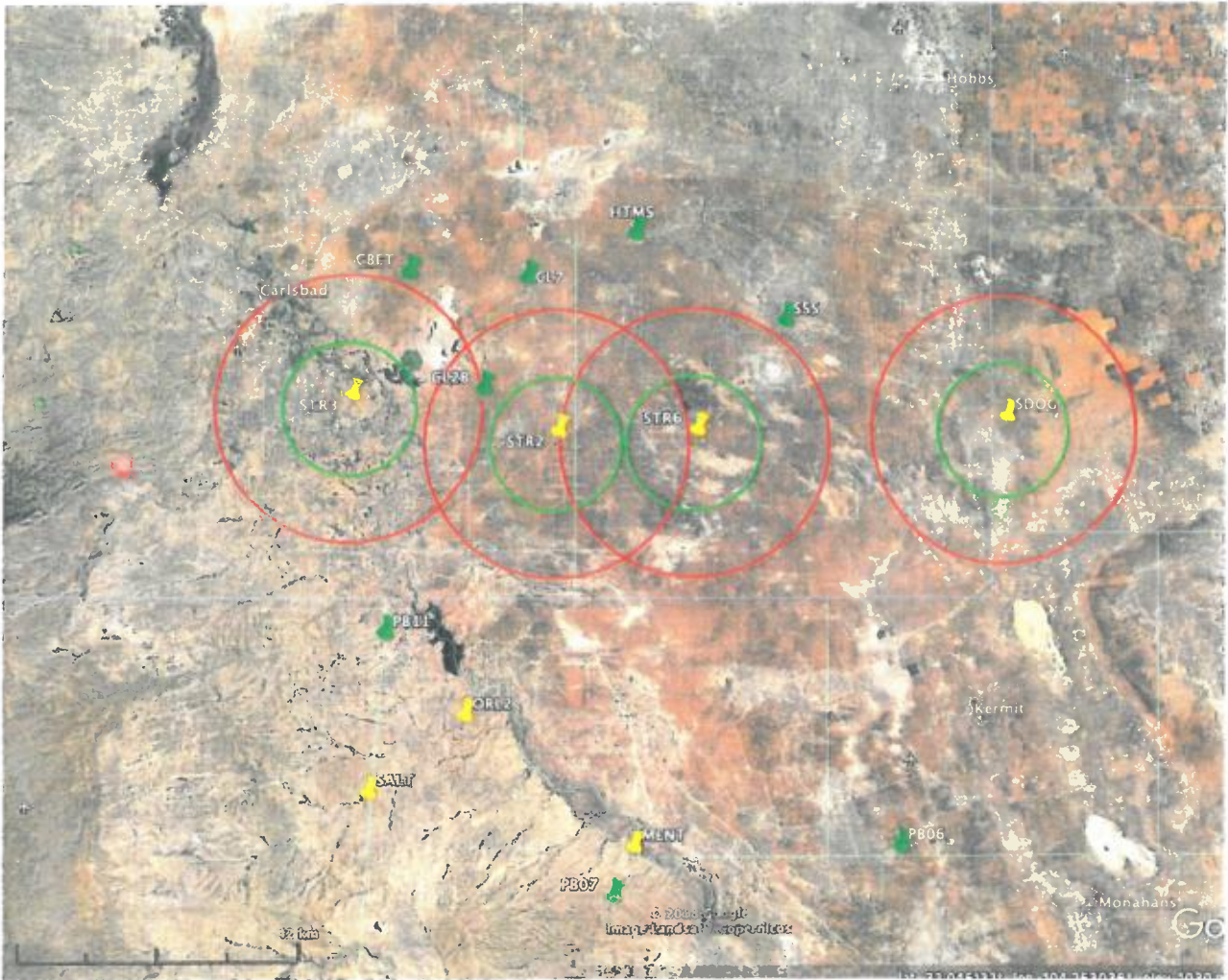
Figure 1. Striker SWD wells seismic station locations and existing NGL-Permian seismic stations (yellow pushpins). Green and red circles around stations show approximate detection levels for ML 1.0 and 1.5, respectively.
