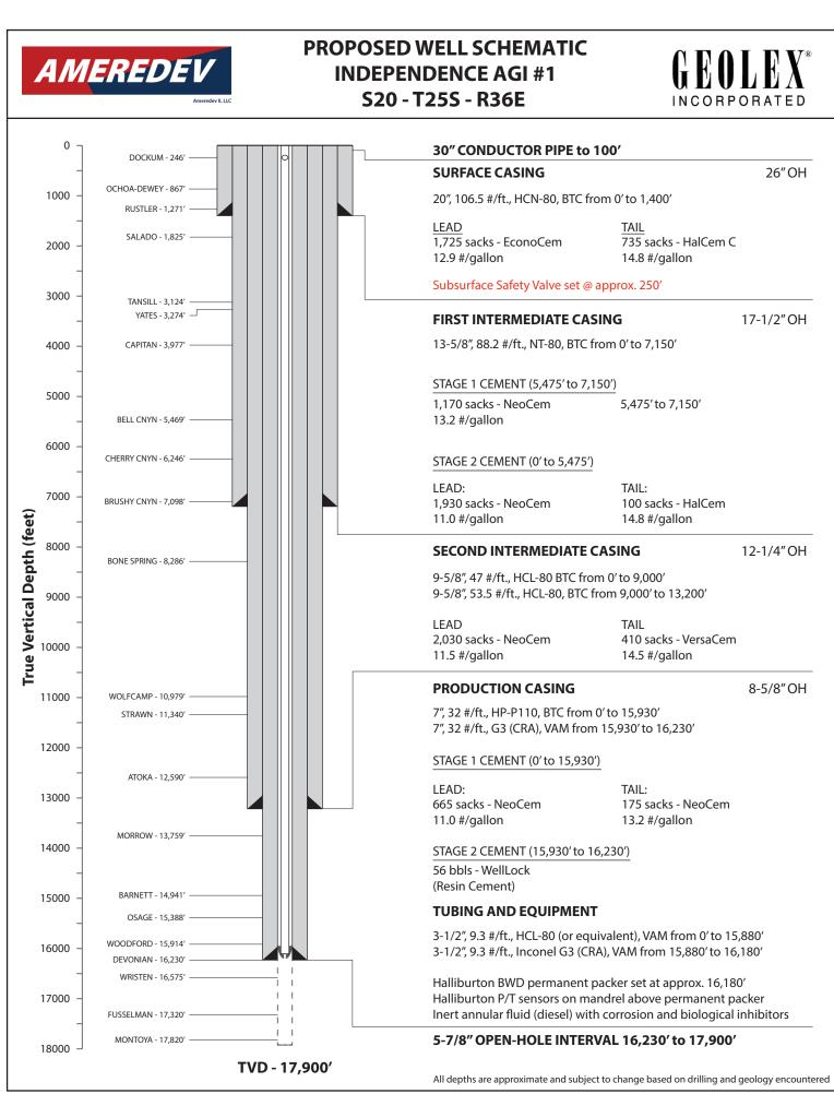
Figure 4. Proposed Independence AGI #1 well schematic Case No. 21381, Sept. 17, 2020 35
