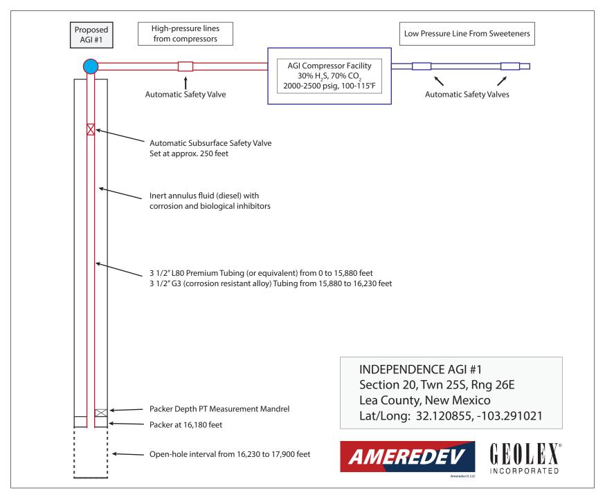
Figure 3. General schematic of surface facilities and proposed Independence AGI #1 Ameredev Operating, LLC Case No. 21381, Sept. 17, 2020
