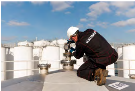
Figure 2.2: Hand gauging with a dipping tape.
