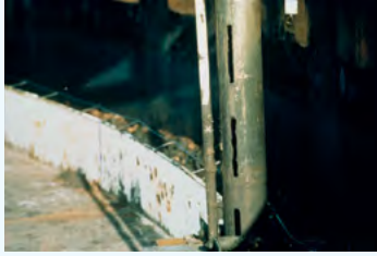
Figure 2.16: Low loss mode radar measurement can be used to virtually eliminate measurement degradation in old still-pipes.
