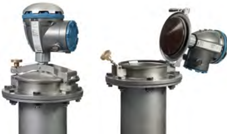
Figure 2.18: Hand dip access in a still-pipe.
