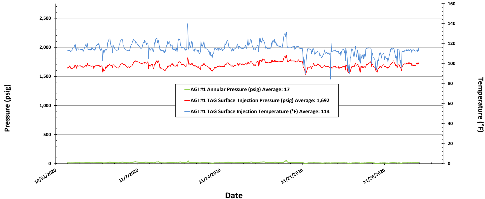
Figure #3: Linam AGI #1 TAG Injection Pressure, Casing Annulus Pressure and TAG Injection Temperature
