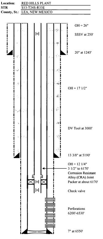
SURFACE CASING 20", 94#/ft, H40, STC at top of Rustler ~ 1245' INTERMEDIATE CASING: 13 3/8", 54.5#/ft, J55, STC at base of salt ~ 5190' PRODUCTION CASING: 7", 26 #/ft, L80, FJ at 6550' TUBING: Subsurface Safety Valve at 250 ft 3 1/2", 9.3#/ft, L80, Premium thread at 6170' PACKER: Permanent Production Packer
