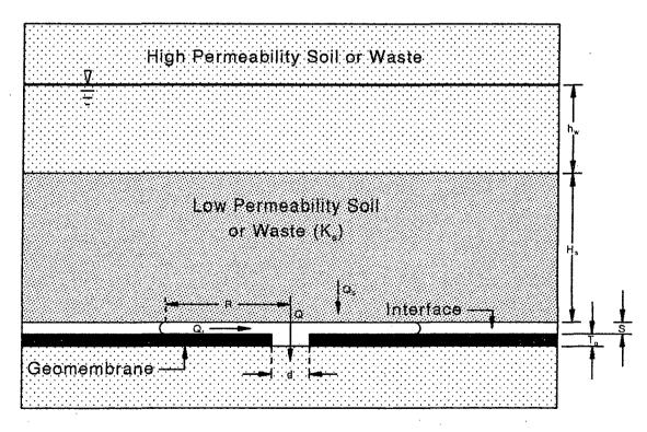
Figure 10. Leakage with Interfacial Flow Above Flawed Geomembrane
