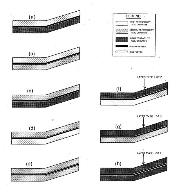
Figure 15. Geomembrane Liner Design Case 5
