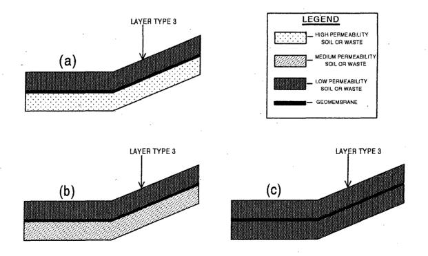
Figure 14. Geomembrane Liner Design Case 4
