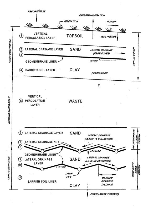
Figure 1. Schematic Profile View of a Typical Hazardous Waste Landfill
