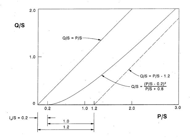
Figure 7. SCS Rainfall-Runoff Relation Normalized on Retention Parameter S
