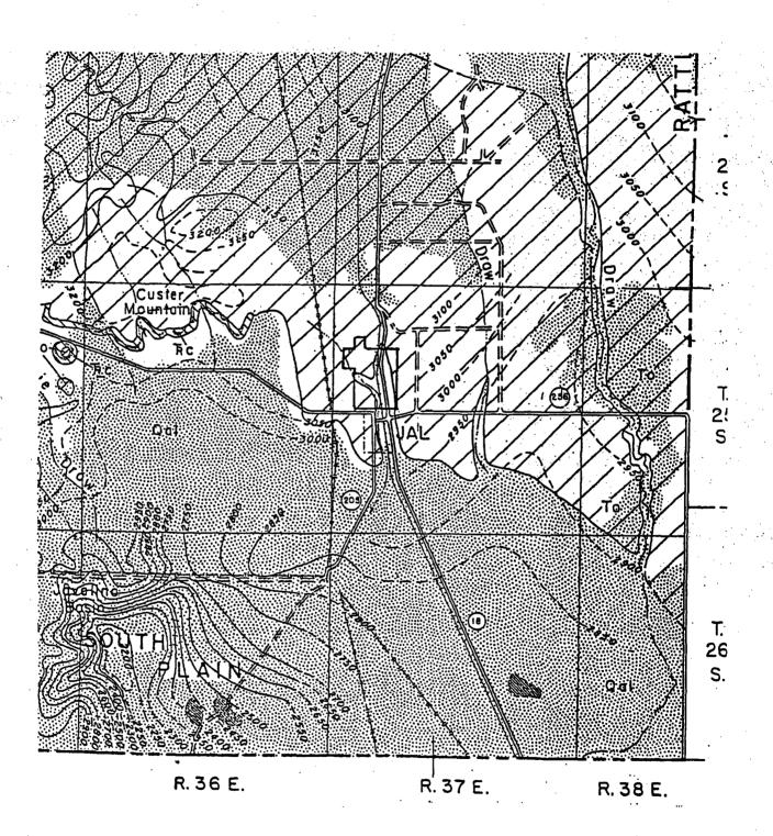
A.6 Copy of a portion of the Ground-Water Map of Southern Lea County, New Mexico showing water-table contours, type of rock from which the water is found, depth to water, depth of well and whether the well is flowing or being pumped.
