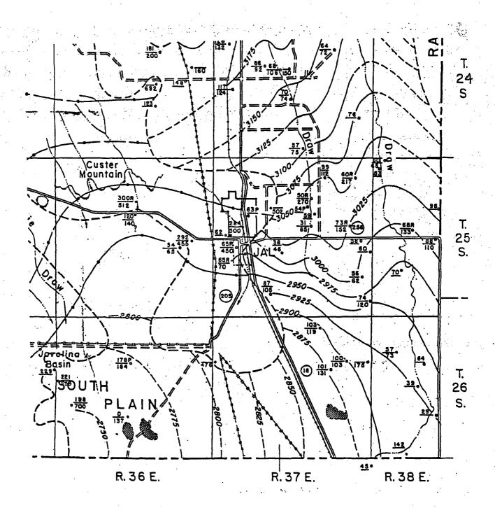
A.7 Well Spot Map showing the location of all known oil and gas wells, water injection wells, tank batteries and pits.
