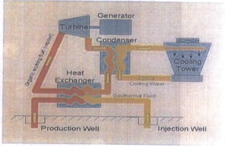
Water is pumped from a geothermal well through a heat exchanger and cooled water is returned to the underground reservoir. A second fluid with a low boiling point is then pumped at a high pressure through the heat exchanger and then vaporizes directing the turbine. It is then condensed by a cold air radiator or cool water and cycles back through the heat exchanger
