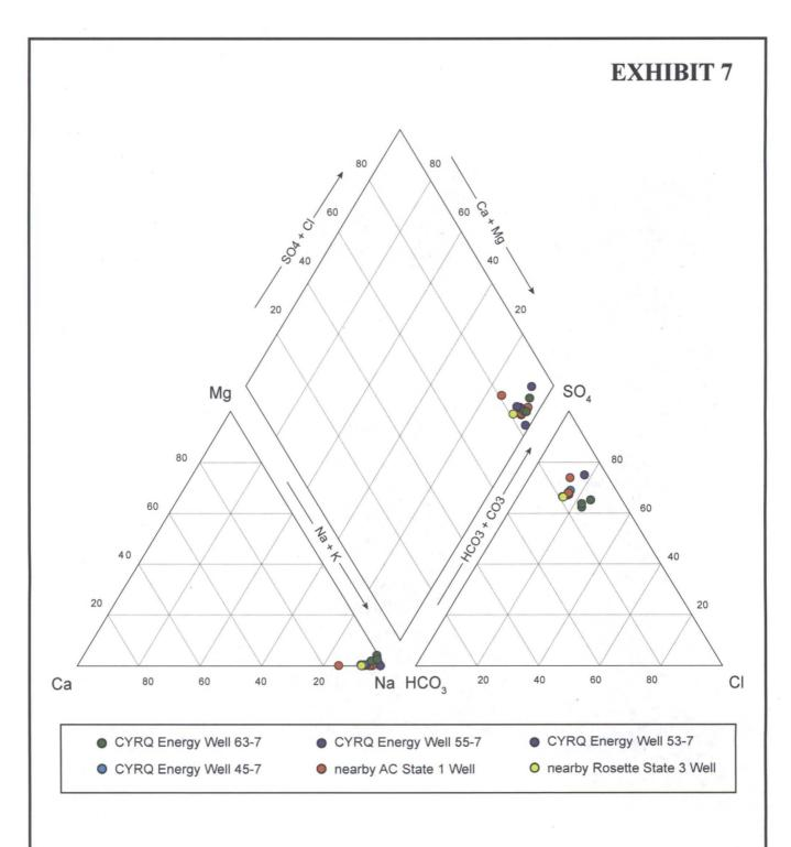
Figure 1. Trilinear diagram (Piper plot, 1944) showing water quality of CYRQ Energy geothermal wells (45-7, 53-7, 55-7, and 63-7) and nearby completed wells, south of Lordsburg, Hidalgo County, New Mexico.
