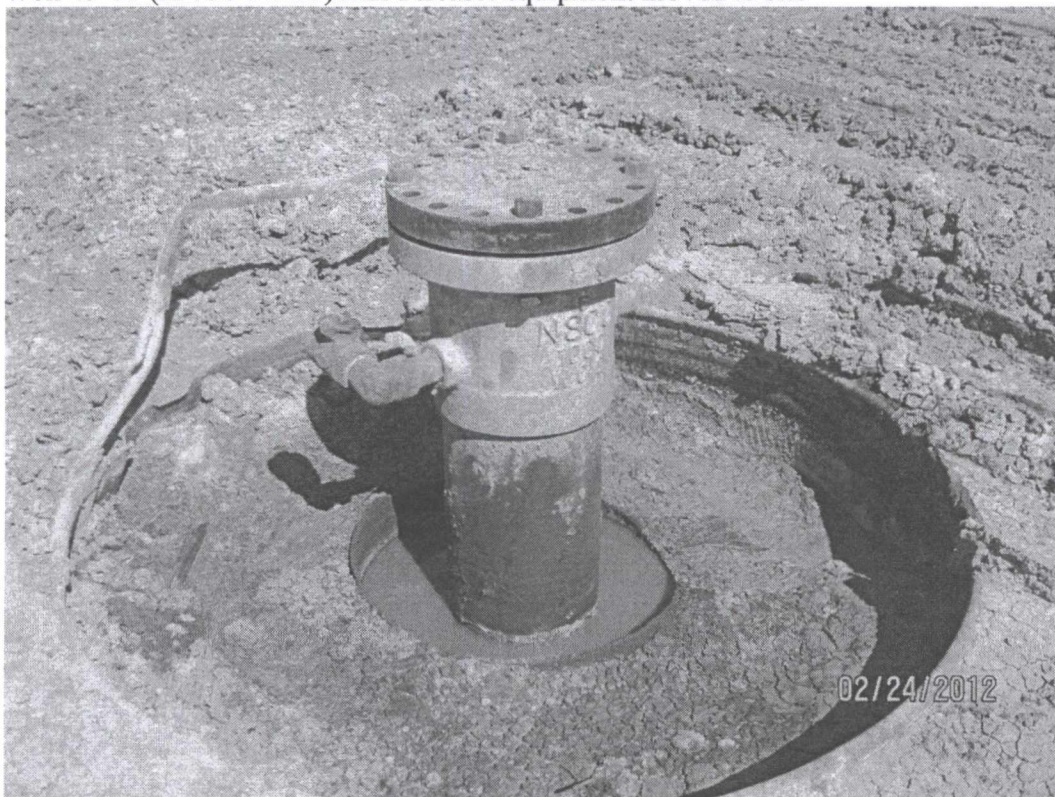
Well 47-07 (A-758-POD6) BLM Lease: well rig removed and well capped (well was recently drilled)
