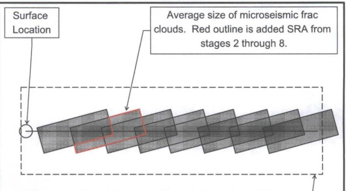
Microseismic data indicated frac clouds averaged 550' of half length, 400' width, and 200' height with orientation of N75°E. Without overlap, stimulated reservoir area (SRA) is 2.3 million sq ft. Proration unit area less setbacks is 6.1 million sq ft. SRA to proration unit ratio is 38%. Loss of SRA due to poor wellbore orientation is 34%.
