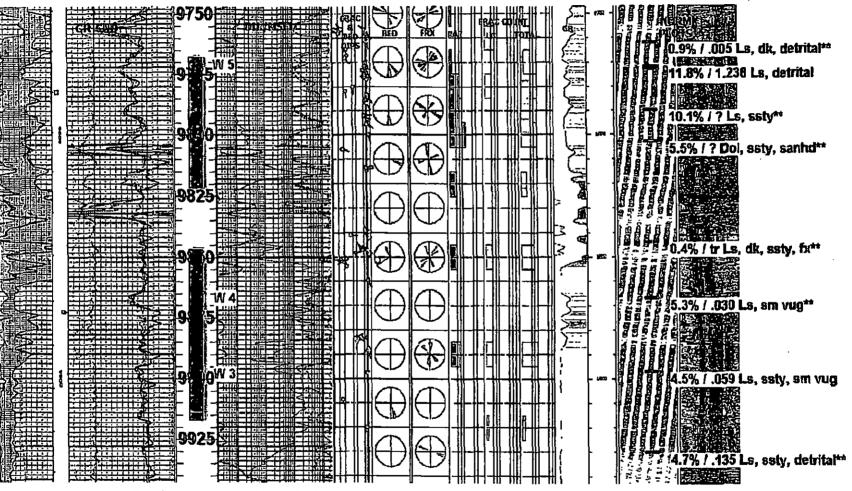
Despite the apparent thinner-bedded nature of the porosity through these intervals, the core results here gave the best, consistent porosity readings over 4%. The FMI shows pervasive fracturing that ties the porous beds together. Zones W5, W4 and W3 should all be perforated by shooting across the entire intervals indicated in blue.
