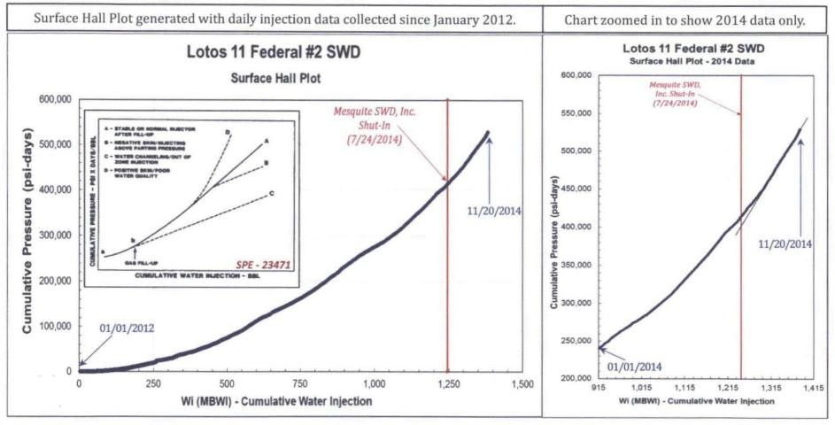
The Surface Hall Plot exhibits a <u>concave upward</u> trend. This trend indicates injection under "normal" conditions, or reduced injectivity over time.
