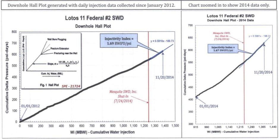
The Downhole Hall Plot primarily exhibits a <u>linear</u> slope, which indicates injection under normal conditions. Injectivity Index is calculated as the inverse of the slope (steeper slope yields smaller I.I.).
