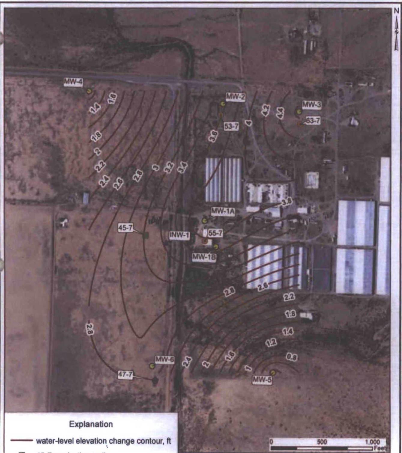
Figure 14. Water-level elevation change in shallow monitoring wells (MW- wells) between December 09, 10, and 11, 2013 (prior to beginning of geothermal operations) and March 17, 2014, Cyrq Energy Lightning Dock Geothermal project. Contour values in feet. Positive value indicates water-level rise.
