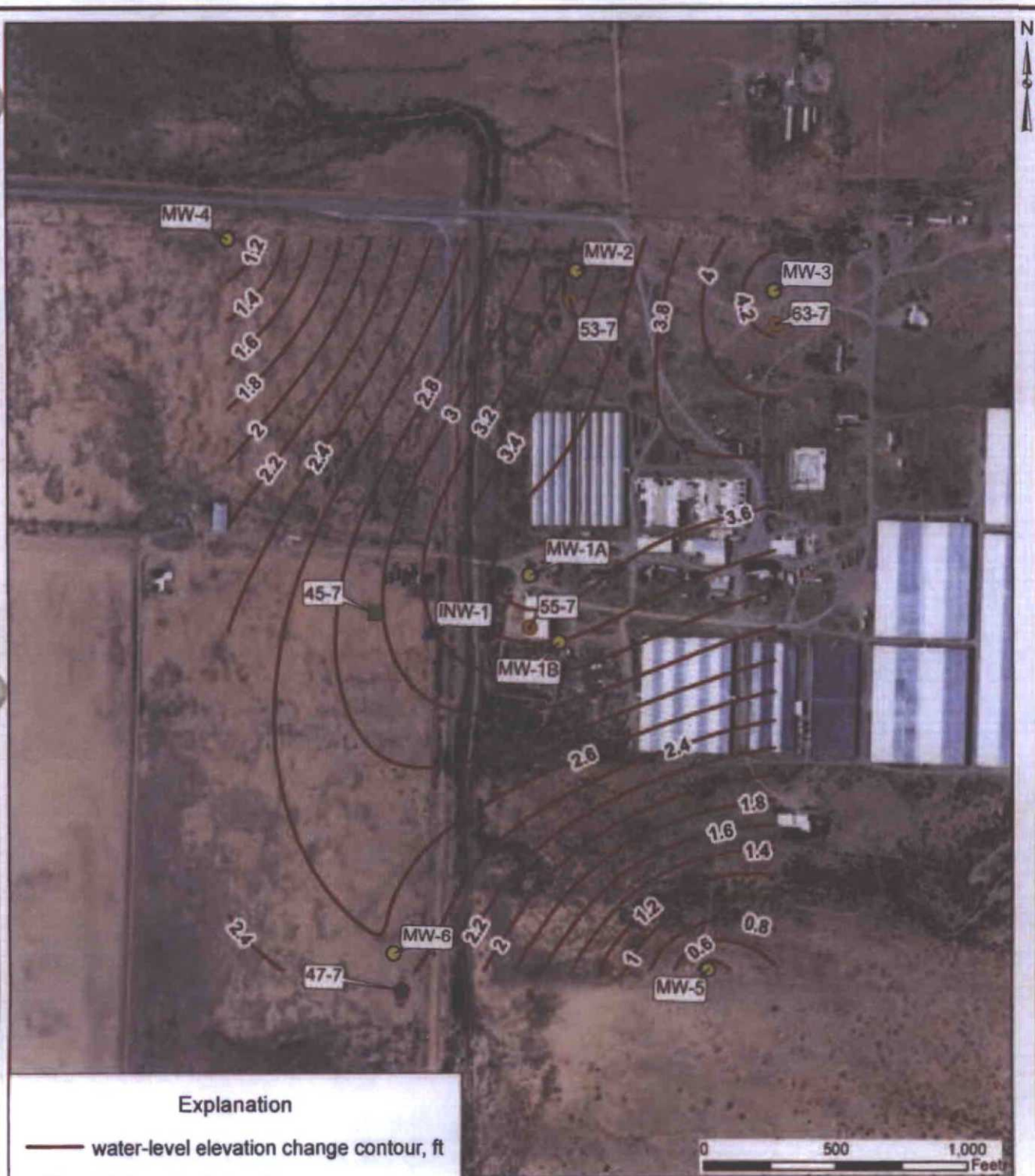
Figure 13. Water-level elevation change in shallow monitoring wells (MW- wells) between December 09, 10, and 11, 2013 (prior to beginning of geothermal operations) and February 22, 2014, Cyrg Energy Lightning Dock Geothermal project. Contour values in feet. Positive value indicates water-level rise.
