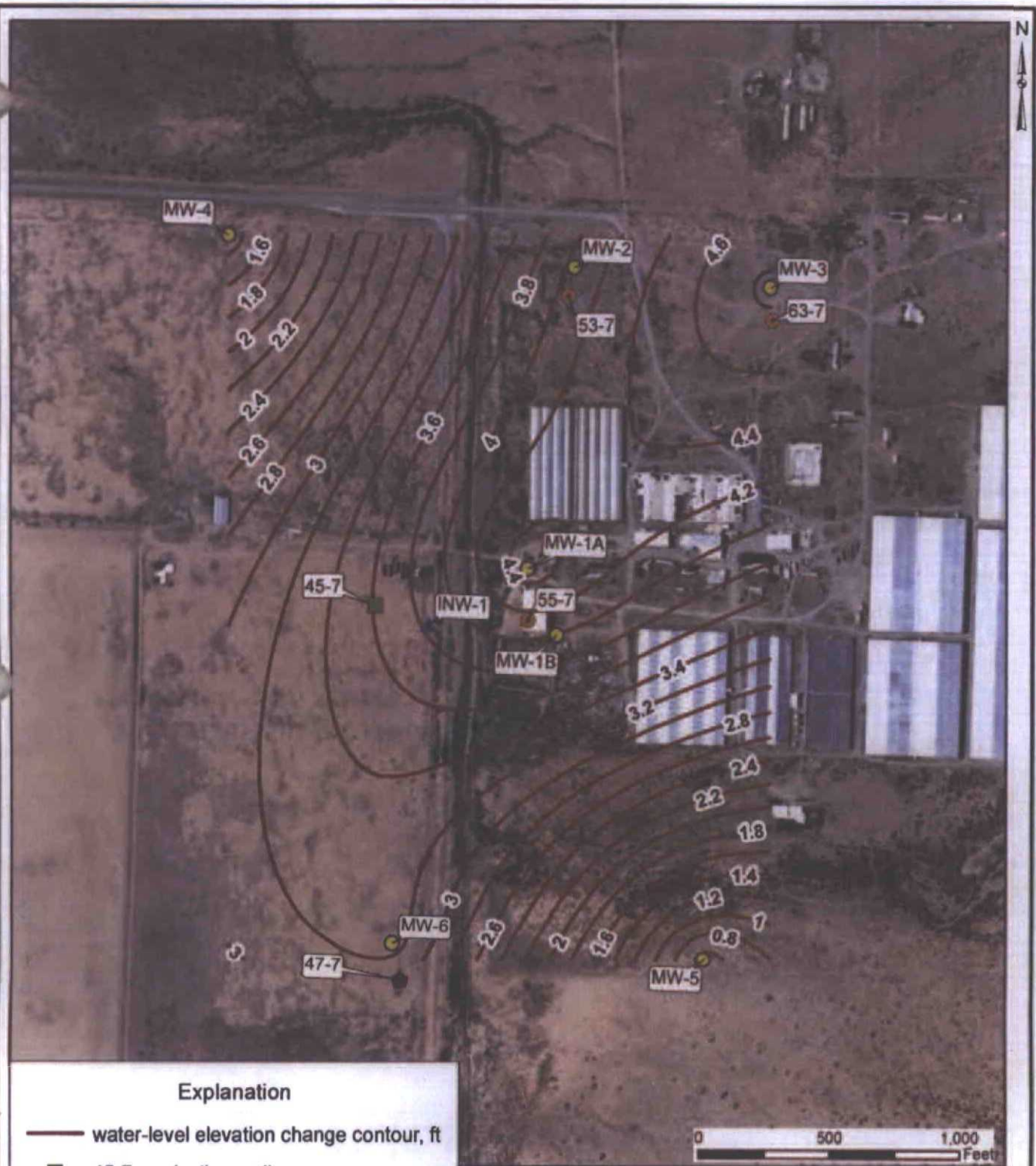
Figure 15. Water-level elevation change in shallow monitoring wells (MW- wells) between December 09, 10, and 11, 2013 (prior to beginning of geothermal operations) and April 17, 2014, Cyrc Energy Lightning Dock Geothermal project. Contour values in feet. Positive value indicates water-level rise.
