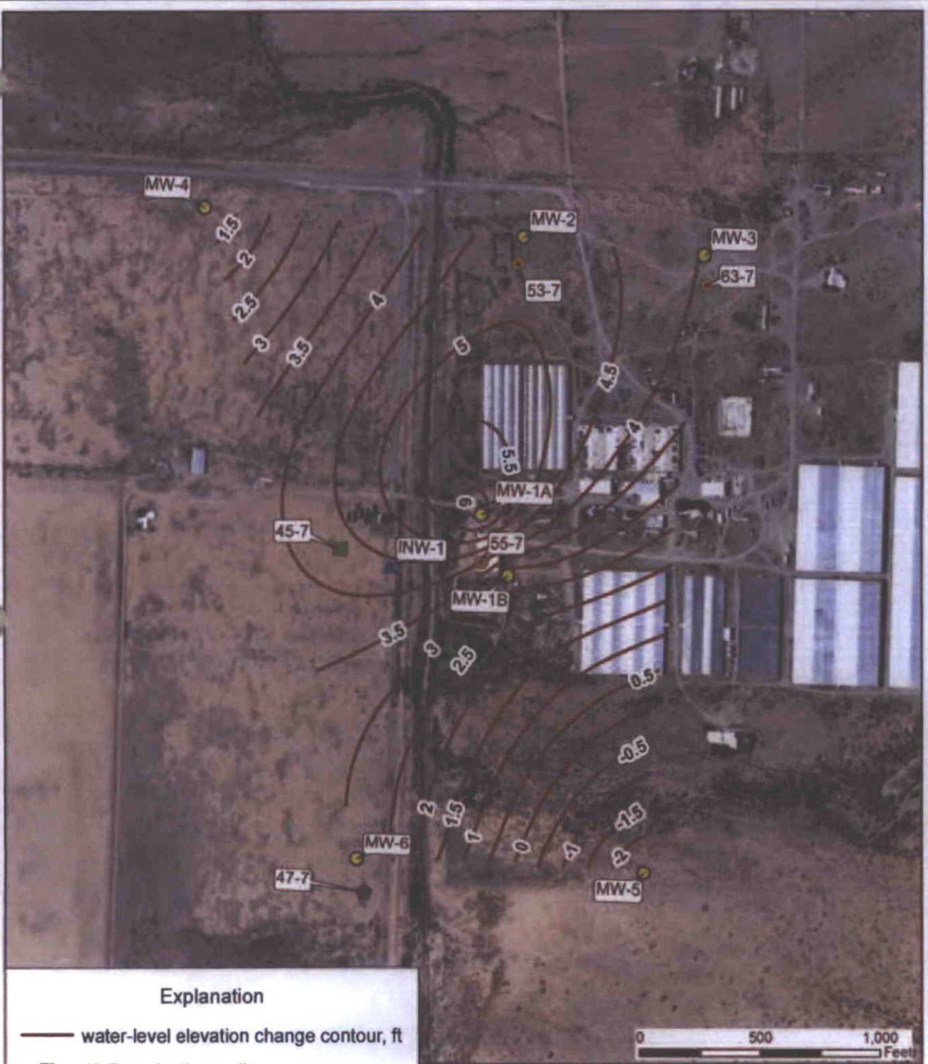
Figure 17. Water-level elevation change in shallow monitoring wells (MW- wells) between December 09, 10, and 11, 2013 (prior to beginning of geothermal operations) and June 19, 2014, Cyrq Energy Lightning Dock Geothermal project. Contour values in feet. Positive value indicates water-level rise.
