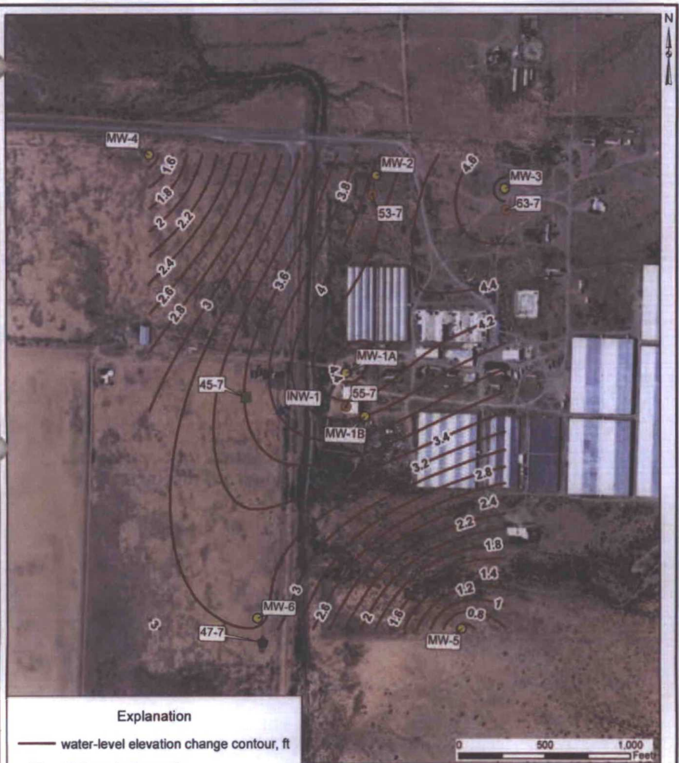
Figure 15. Water-level elevation change in shallow monitoring wells (MW- wells) between December 09, 10, and 11, 2013 (prior to beginning of geothermal operations) and April 17, 2014, Cyrg Energy Lightning Dock Geothermal project. Contour values in feet. Positive value indicates water-level rise.
