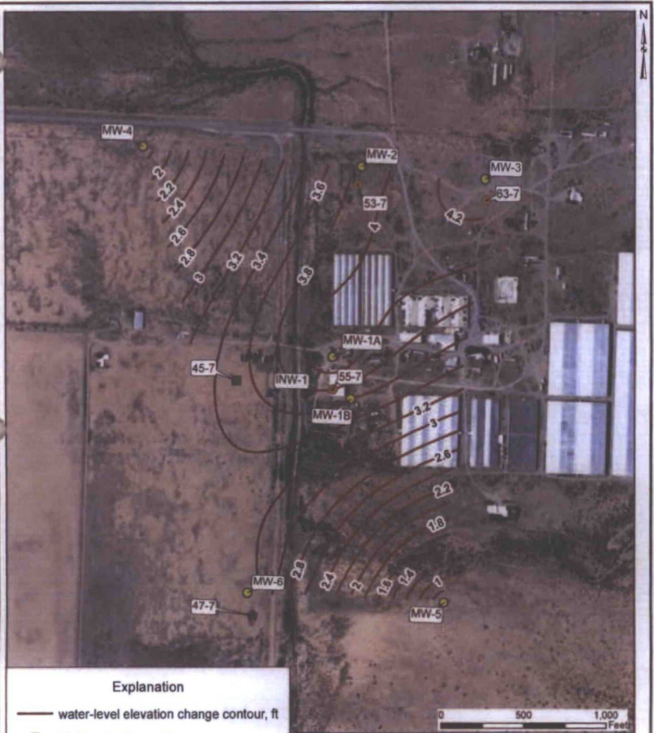
Figure 16. Water-level elevation change in shallow monitoring wells (MW- wells) between December 09, 10, and 11, 2013 (prior to beginning of geothermal operations) and May 11, 2014, Cyrc Energy Lightning Dock Geothermal project. Contour values in feet. Positive value indicates water-level rise.
