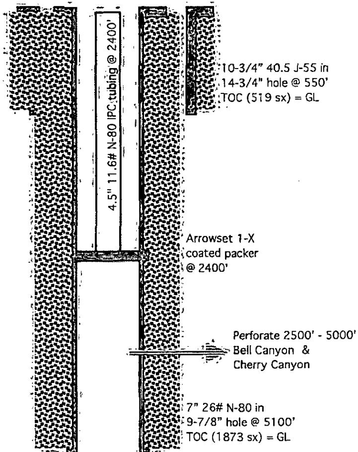
WELL CONSTRUCTION DATASurface Casing
