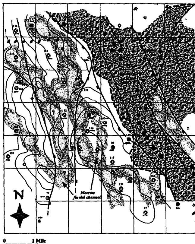
Figure 6. Structure of the top of the Morrow clastics (C. I. = 100 feet) in eastern Lea County, New Mexico, showing the effects of inhibited Morrow deposition due to active tectonic movements and complete removal of remaining Morrow sediments during later widespread exposure and erosion. Major fluvial channel fairways are shown, locally terminating against younger faults. Variable thicknesses of the Morrow clastic section are shown by each deep well.
