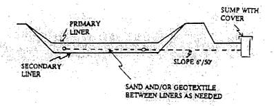
NOTE: SKIMMER POND TO HAVE SEPARATE LEAK DETECTION SYSTEM AND SUMP.
