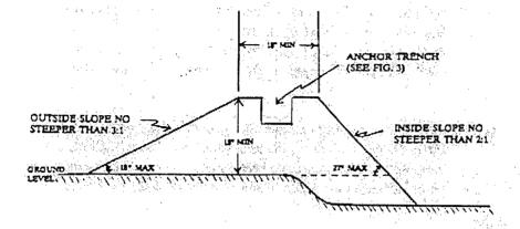
NOTE: LEVEE TO BE CONSTRUCTED IN A MANNER SUCH THAT DESIGN COMPACTION AND DIMENSIONS PROVIDE FOR A MINIMUM SAFETY FACTOR OF TWO FOR FORCES ACTING AGAINST THE
