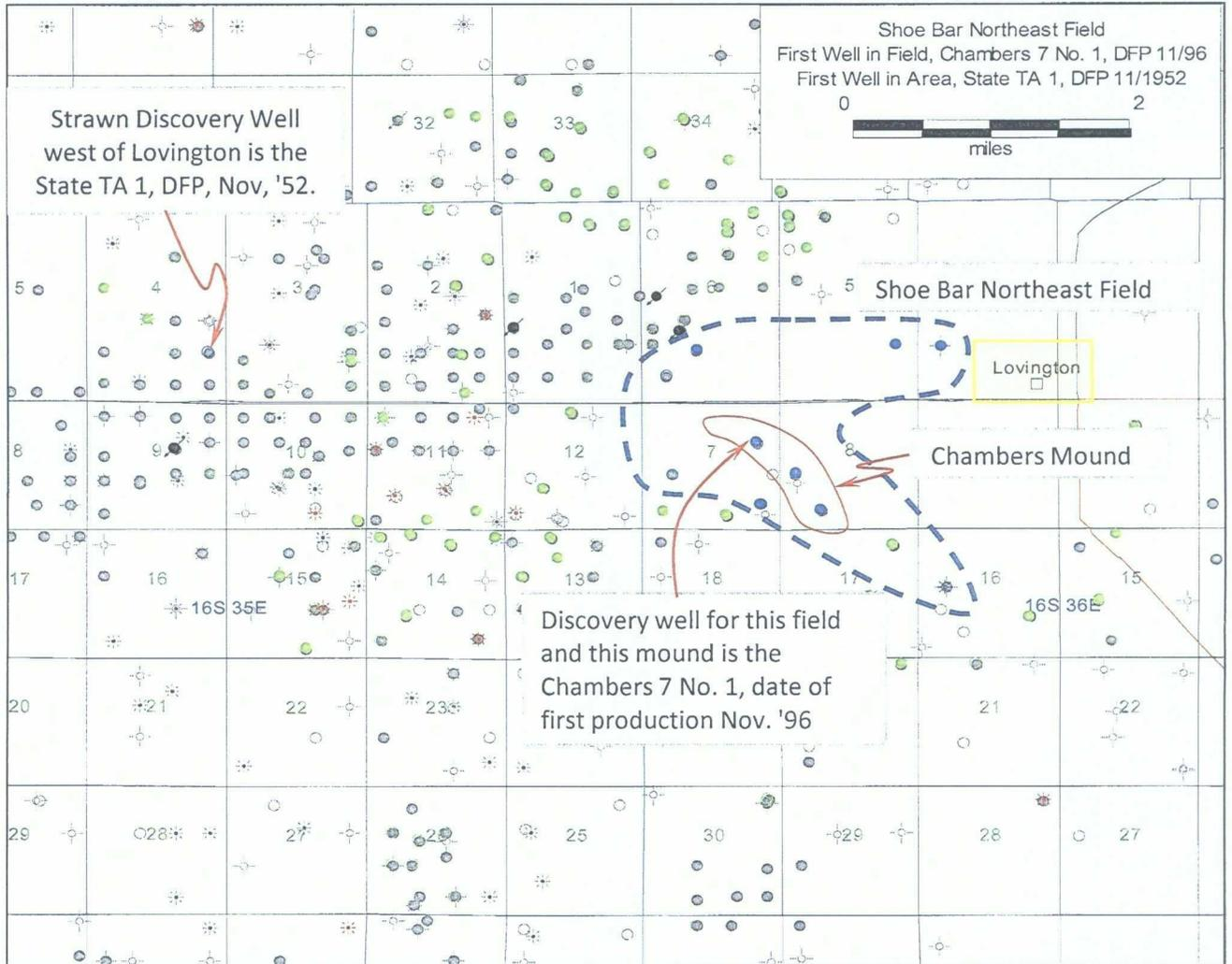
The group of Strawn wells known as the Shoe Bar Northeast Field is shown above. The field contains 10 Strawn completions in portions of six sections. The field lies generally to the southwest of Lovington, New Mexico.
