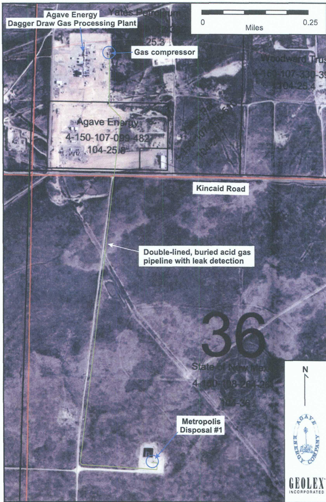
Figure 2: General Diagram of Agave Dagger Draw Gas Plant and Location of Pipeline Connecting the Plant with the Metropolis Disposal #1 Well
