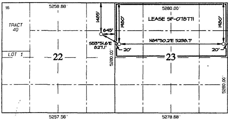
THE HORIZONTAL LATERAL REPRESENTED ON THIS PLAT CORRESPONDS TO THE BLACK SEGMENT WHICH VARIES IN THE ELEVATION FROM 6891.0' AT THE POINT-OF-ENTRY TO 6749.0' AT THE END-OF-LATERAL.
