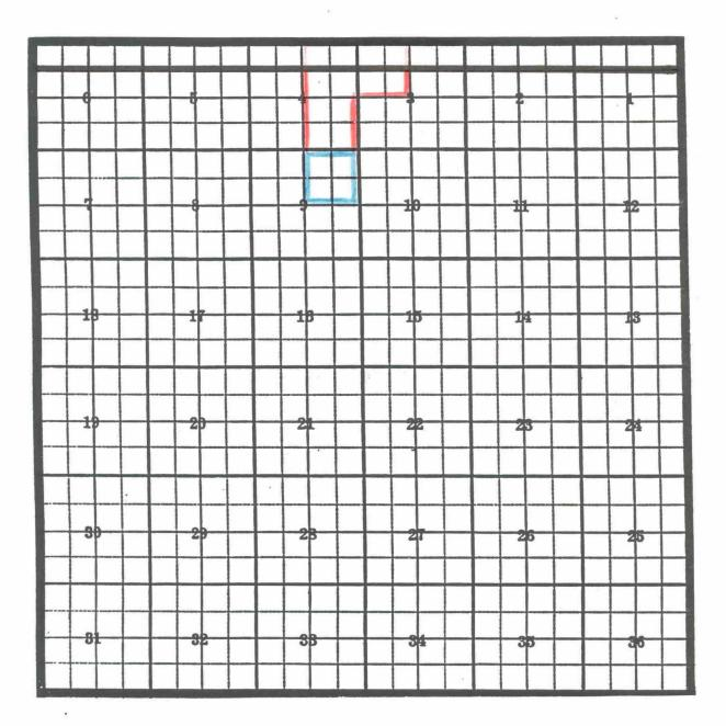
PURPOSE: One completed oil well capable of producing. Marbob Energy Corporation, Rooster Cogburn Fee #1 Unit G , Sec. 9, T-11-S, R-28-E, NMPM. Completed 9/28/96 in the Devonian formation. Top of perforations are at 7076 feet.
