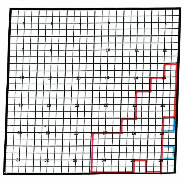
PURPOSE: Two completed oil wells capable of producing. (1) Devon Energy Corporation, Todd "25B" Federal #2 Unit B, Sec. 25, T.23S., R.31E., NMPM. Completed 12-14-96 in the Delaware formation. Top of perforations are at 7125 feet.
