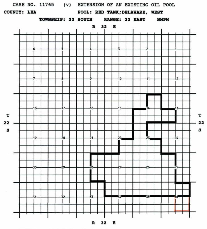
PURPOSE: One completed oil well capable of producing. BURLINGTON RESOURCES OIL AND GAS COMPANY, MULE DEER 36 STATE # 7, P-36-T22S-R32E, completed 02/02/1997, in the Delaware Formation, top perfs 8559 ft.
