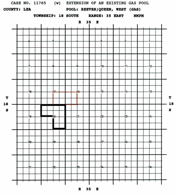
PURPOSE: One completed gas well capable of producing. MARALO INC, MARALO SV 16 STATE COM # 1, L-16-T18S-R35E, completed 12/22/1995, in the Queen Formation, top perfs 4340 ft.
