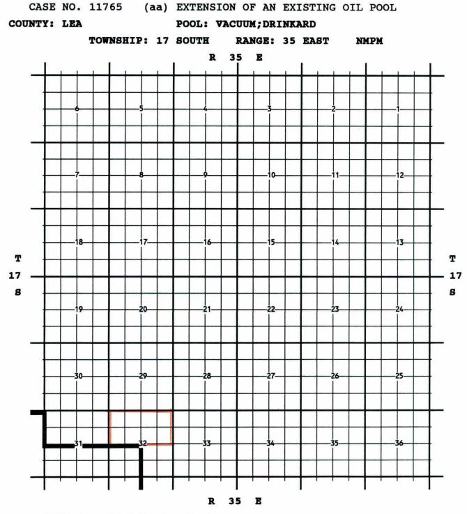
PURPOSE: One completed oil well capable of producing. SHELL WESTERN E & P INC, HOOVER 32 # 1, H-32-T17S-R35E, completed 12/12/1996, in the Drinkard Formation, top perfs 7624 ft.
