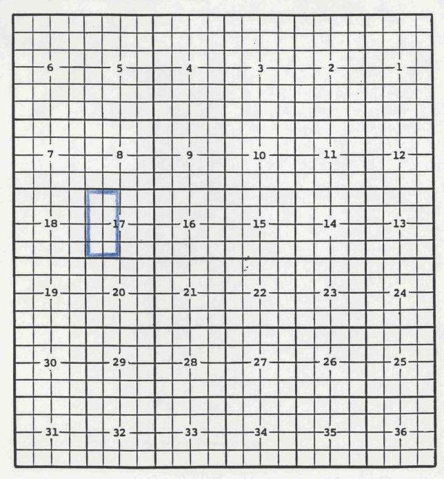
PURPOSE: One completed gas well capable of producing. Marbob Energy Corporation, Como Fee #1 Unit F, Sec. 17, T.21S., R.25E., NMPM. Completed 5-02-97 in the Morrow formation. Top of perforations are at 10259 feet.
