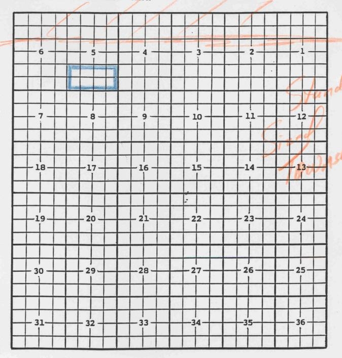
PURPOSE: One completed gas well capable of producing. Yates Petroleum Corporation, Federal "HQ" #1 Unit N, Sec. 5, T.21S., R22E., NMPM Completed 7-22-88 in the Strawn formation. Top of perforations are at 7538 feet.
