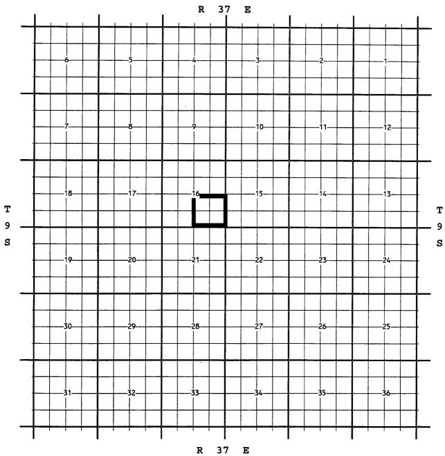
PURPOSE: One completed oil well capable of producing. COBRA OIL & GAS CORPORATION, STATE 16 # 1-Y, P-16-T9S-R37E, completed 10/05/1997, in the Devonian Formation, top perfs 12551 ft.
