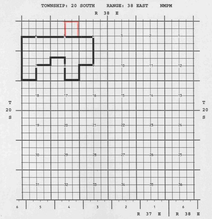
PURPOSE: One completed oil well capable of producing. CROSS TIMBERS OPER CO, DEWEY # 2, G-5-T2OS-R38E, completed 12/12/1997, in the Drinkard Formation, top perfs 6907 ft.
