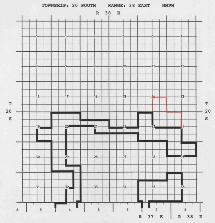
PURPOSE: One completed oil well capable of producing. COLLINS & WARE INC, M & M # 2, F-24-T2OS-R38E, completed 07/18/1997, in the Blinebry Formation, top perfs 5966 ft.
