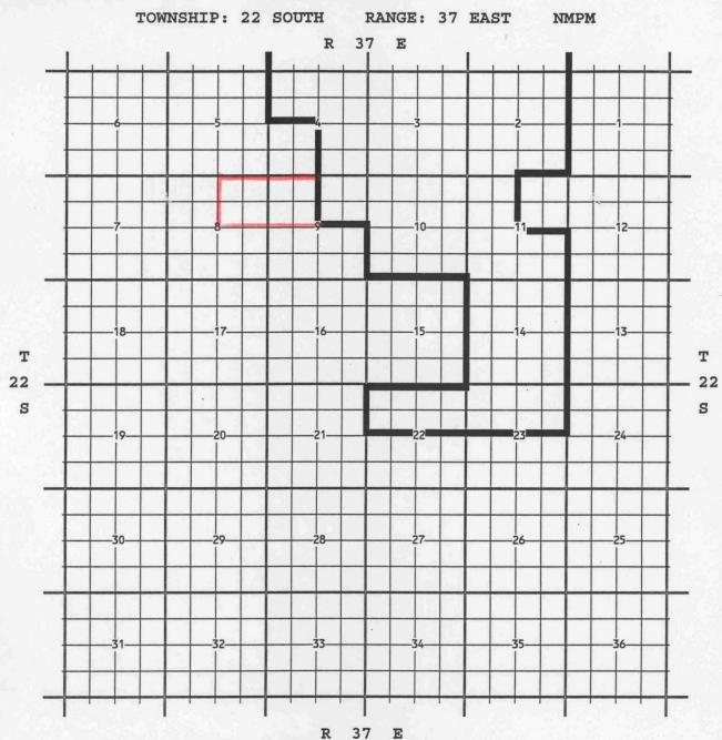
PURPOSE: One completed oil well capable of producing. ZIA ENERGY INC, GRIZZELL B # 4, G-8-T22S-R37E, completed 03/22/1998, in the Abo Formation, top perfs 7100 ft.
