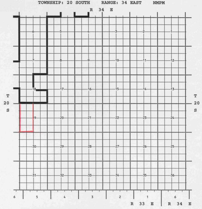
PURPOSE: One completed gas well capable of producing. SANTA FE ENERGY RESOURCES INC, TOPAZ 19 FED COM # 1, N-19-T20S-R34E, completed 05/22/1998, in the Morrow Formation, top perfs 13686 ft.
