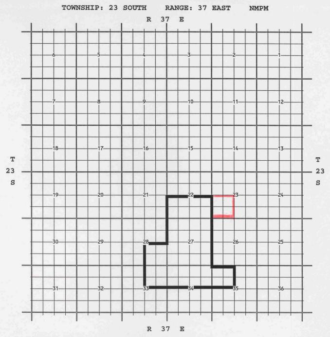
PURPOSE: One completed oil well capable of producing. ENRON OIL & GAS CO, HUNT 23 # 1, N-23-T23S-R37E, completed 06/15/1998, in the Ellenburger Formation, top perfs 10925 ft.
