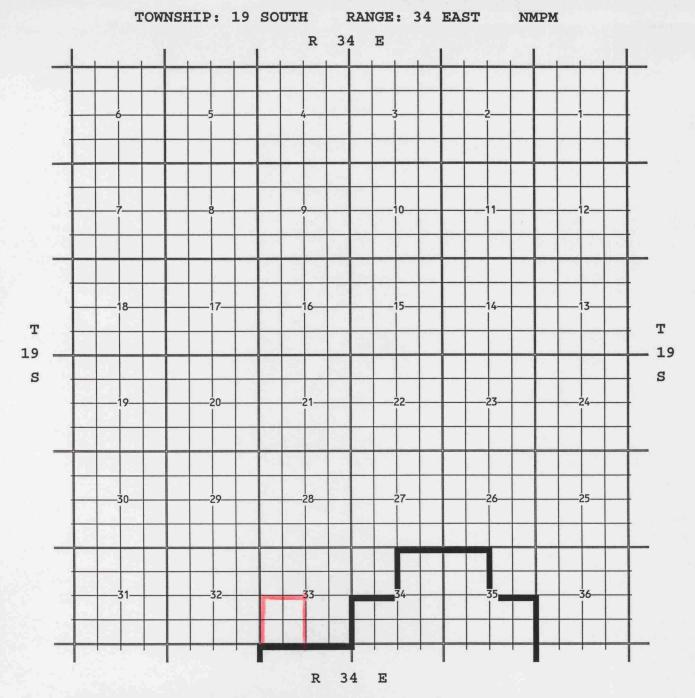
PURPOSE: One completed oil well capable of producing. READ & STEVENS INC, PEARL 33 FEDERAL # 1, N-33-T19S-R34E, completed 01/17/1998, in the Delaware Formation, top perfs 7038 ft.
