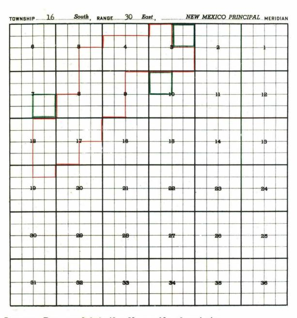
Purpose: Three completed oil wells capable of producing. Leonard Oil Co.-Federal Hagerty #6 in Unit P of Section 7-16-30 Completed in Premier 12-13-58. Depth to Casing Shoe 2703'. Shell Oil Co.-Little Lucky Lake Unit #3 in Unit J of Sec. 3-16-30 UNADVERTISED: Completed in Grayburg 1-25-59. Top of perforations 2832.
