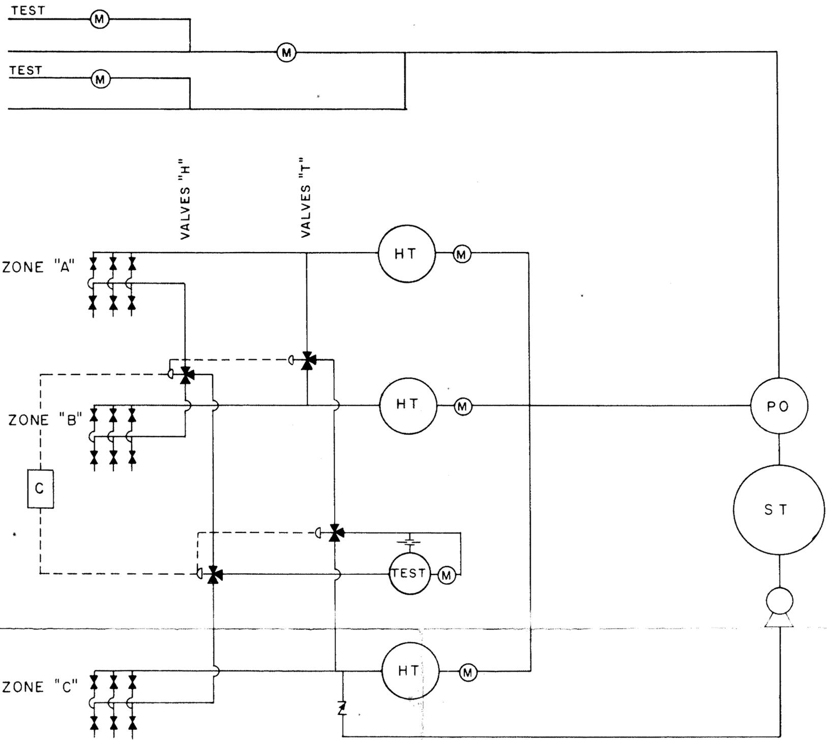
1. Automatic well test header valves on individual well flowlines may be substituted for valve "H". Interlocking control as shown would then be required between each valve on the manifold and the respective valve "T".
