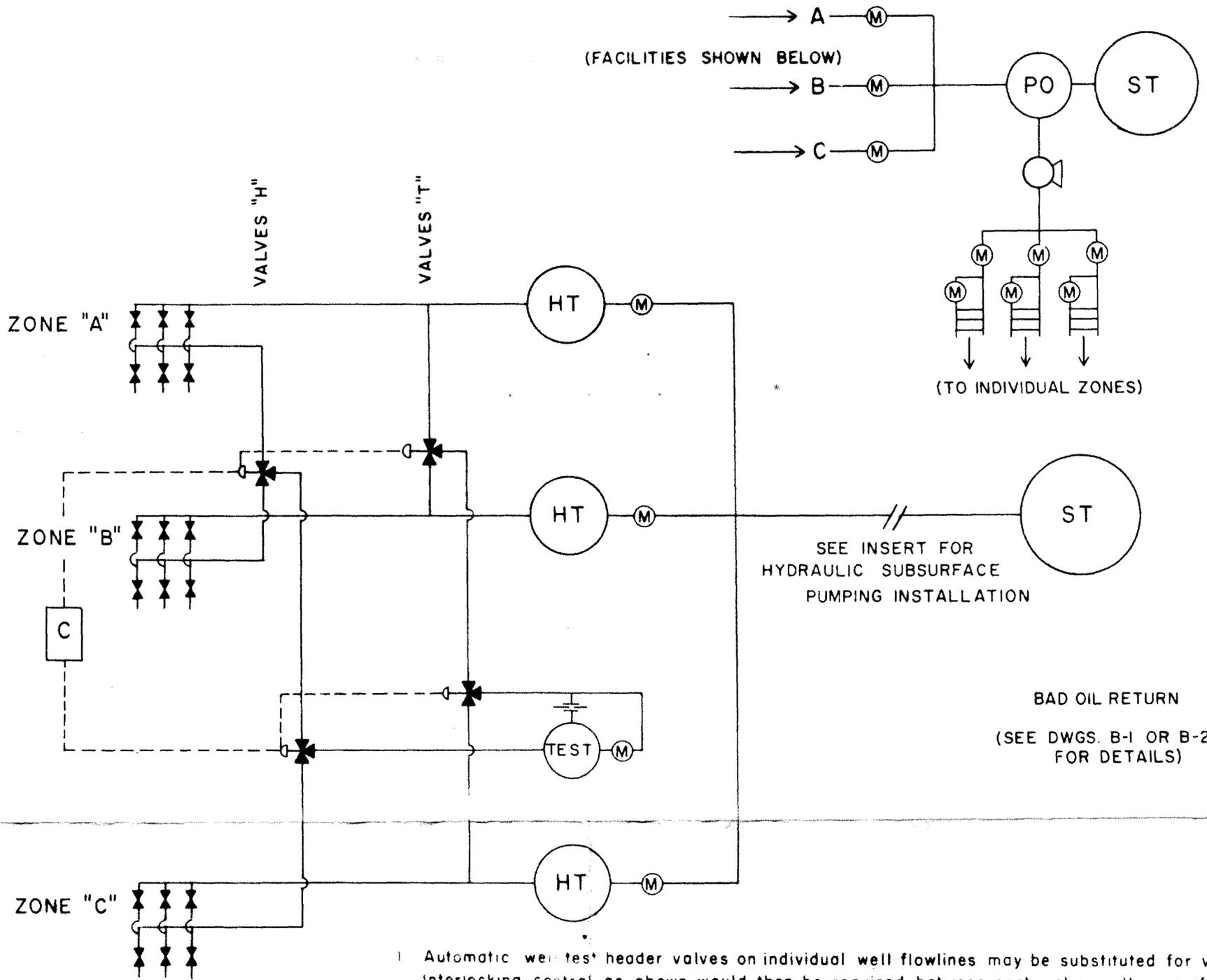
1. Automatic well test header valves on individual well flowlines may be substituted for valve "H" interlocking control as shown would then be required between each valve on the manifold and the respective valve "T".
