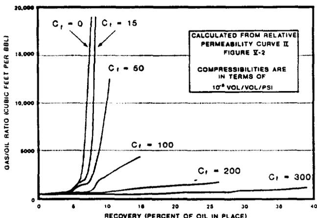
**Figure 5-4.** Solution gas drive recovery using relative permeability curve II and various formation compressibilities. Note extreme range of recoveries for the different compressibilities.
