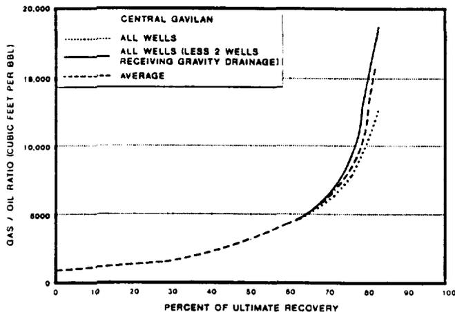
Figure 5-6. GOR history of central Gavilan from field data. Average curve is used in making comparisons of calculated histories with field performance. Percent of ultimate recovery is based on cumulative recovery of production below maximum assumed bubble point pressure of 1660 psi.
