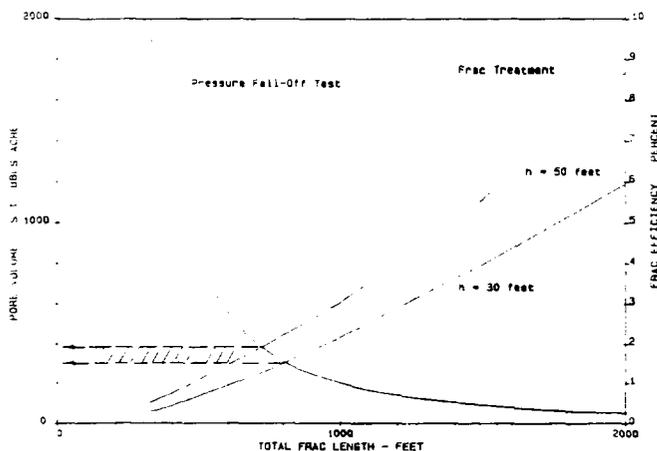
**Figure 3-5.** Combination of Figures 3-3 and 3-4 using arbitrarily selected maximum ordinate of 2000 stock tank barrels per acre for location of data of pressure fall-off test. Interpreted frac length 700 to 800 ft. Pore volume of well's low capacity fracture block approximately 300 to 400 barrels per acre using KGD method of hydraulic fracture analysis.
