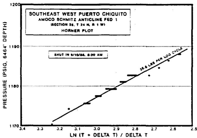
**Figure 6-3.** Plot of portion of build-up of Figure 6-1 greatly expanded to show "late-time" straight line slope of approximately 26 lb per log cycle, evidencing presence of high capacity fracture in well's immediate drainage area.
