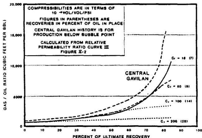
Figure 5-9. Calculated solution gas drive recoveries using  $k_g/k_o$  curve III of Figure 5-2 and various formation compressibilities. Note low value of maximum GORs for curves with  $C_f$  of  $50 \times 10^{-6}$  and greater.
