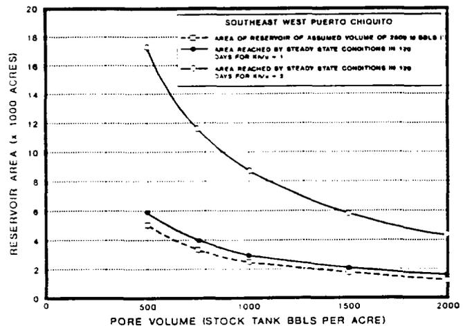
Figure 6-6. Plot showing reservoir area covering volume of 2.5 million bbl as dependent on per acre pore volume along with the concurrent area that could be reached by steady state conditions for the transmissibilities shown.
