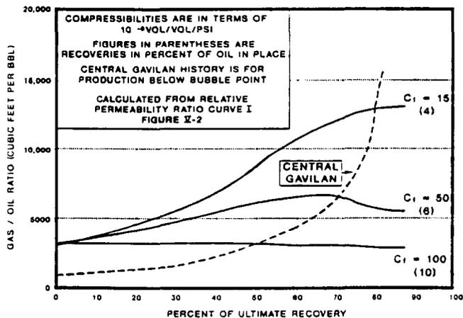
Figure 5-7. Calculated solution gas drive recoveries using  $k_g/k_o$  curve I of Figure 5-2 and various formation compressibilities. Histories are GOR versus ultimate recovery. Note failure of calculated curves to "match" field performance.
