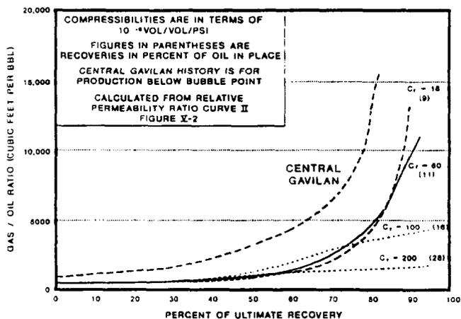
Figure 5-8. Calculated solution gas drive recoveries using  $k_g/k_o$  curve II of Figure 5-2 and various formation compressibilities. Note these curves fall below that of field performance. Note divergence from field data of curves for  $C_f = 100$  and  $200 \times 10^{-6}$ .
