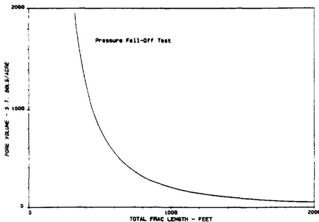
**Figure 3-3.** Relation of unit pore volume (stock tank barrels per acre) to fracture length of hydraulically induced fracture of the COU A-14 well determined from pressure fall-off test shown in Figure 3-2.
