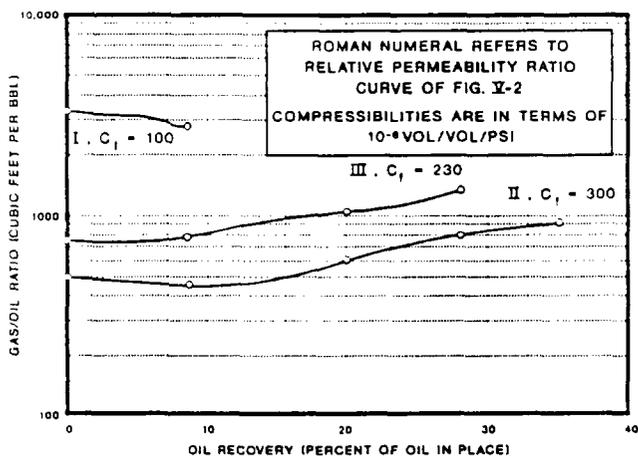
**Figure 5-3.** Solution gas drive GOR histories using "critical" formation compressibility. Note high recoveries for  $k_g/k_o$  curves II and III and that shape of all GOR curves bears no resemblance to that of typical solution gas drive reservoirs.
