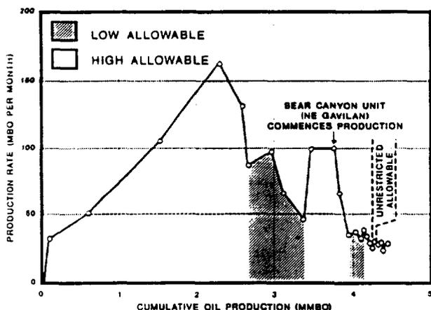
**Figure 5-5.** Plot of production rate versus cumulative recovery for central Gavilan. Periods of high and low allowables are identified along with one period of unrestricted allowable. Economic ultimate recovery of 5 million bbl estimated from this plot.
