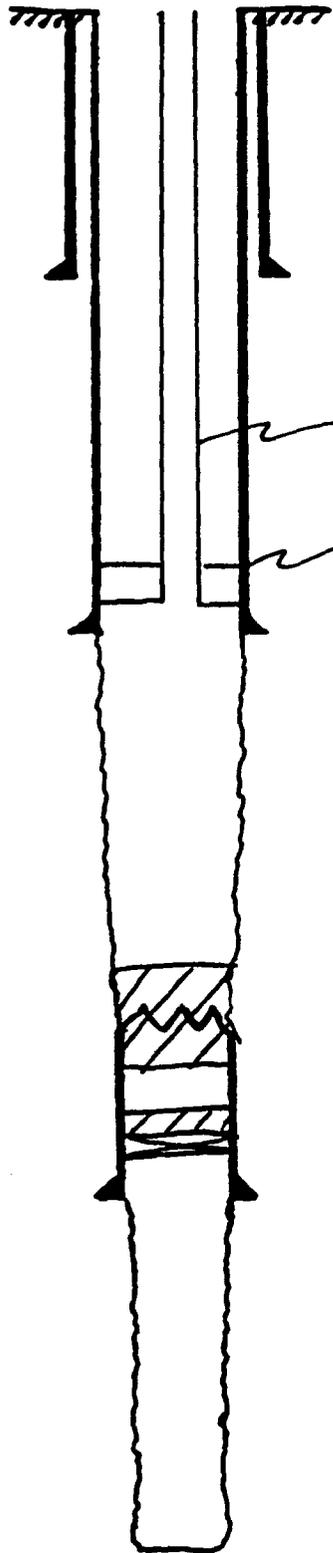
13<sup>3</sup>/<sub>8</sub>" casing set at 303' with 350 sx of \_\_\_\_\_ cement
