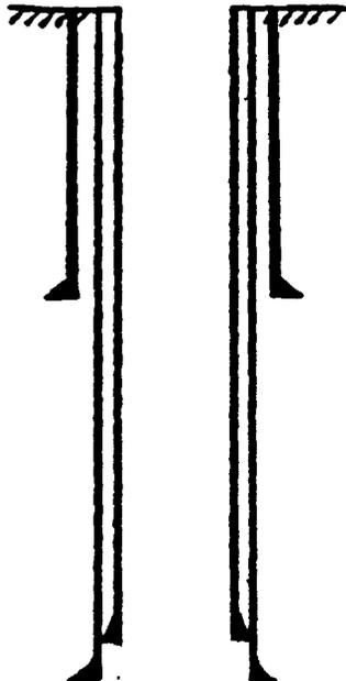
13 3/8" casing set at 293' with 350 sx of \_\_\_\_\_ cement
