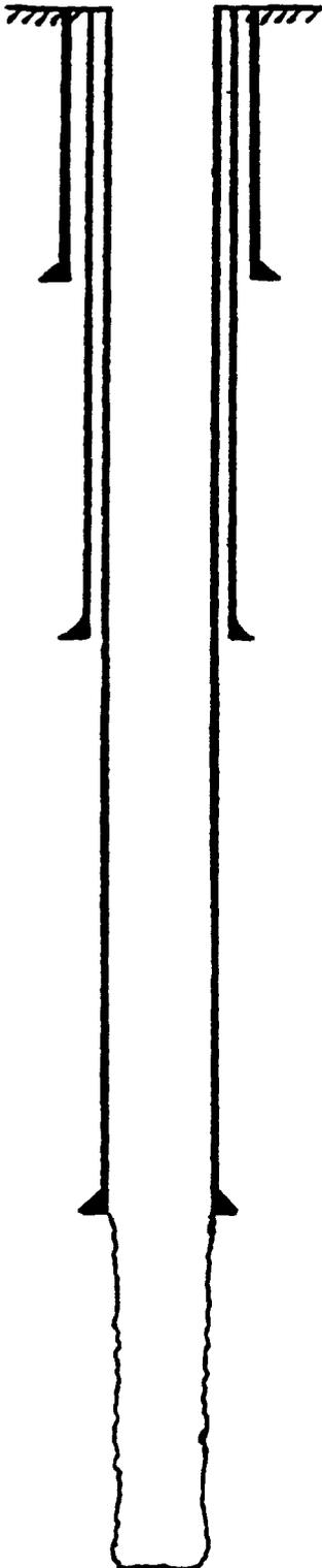
13 3/8" casing set at 365' with 425 sx of \_\_\_\_\_ cemen.
