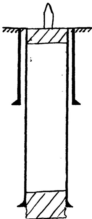
$13\frac{3}{8}$ " casing set at 303' with 350 sx of \_\_\_\_\_ cemen
