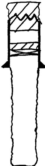
$5\frac{1}{2}$ " casing set at 12203' with 500 sx of \_\_\_\_\_ cemen
