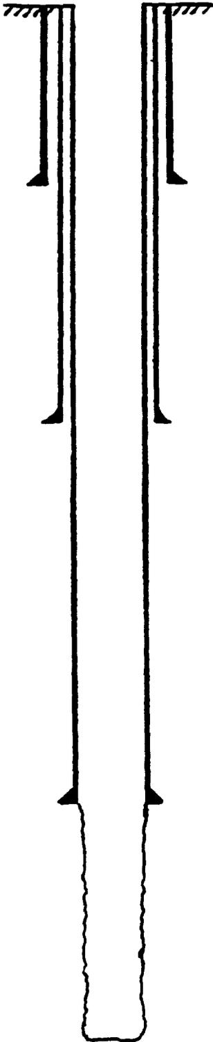
12 3/4" casing set at 365' with 450 sx of \_\_\_\_\_ ceme
