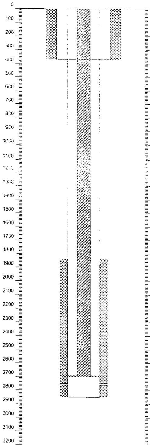
370'. 8-5/8" 24# J-55 CASING, CEMENTED WITH 375 SACKS, CIRCULATED
