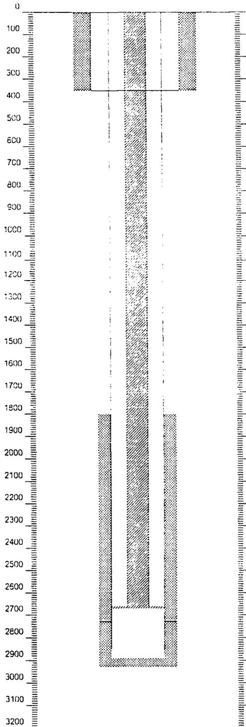
265', 8-5/8" 24# J-55 CASING, CEMENTED WITH 265 SACKS, CIRCULATED
