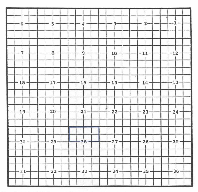
PURPOSE: One completed gas well capable of producing. Collins and Ware, Inc., Happy Valley Federal Com #1 Unit G, Sec.28, T.22S., R.26E., NMPM. Completed 3-8-93 in the Wolfcamp formation. Top of perforations are at 9571 feet.
