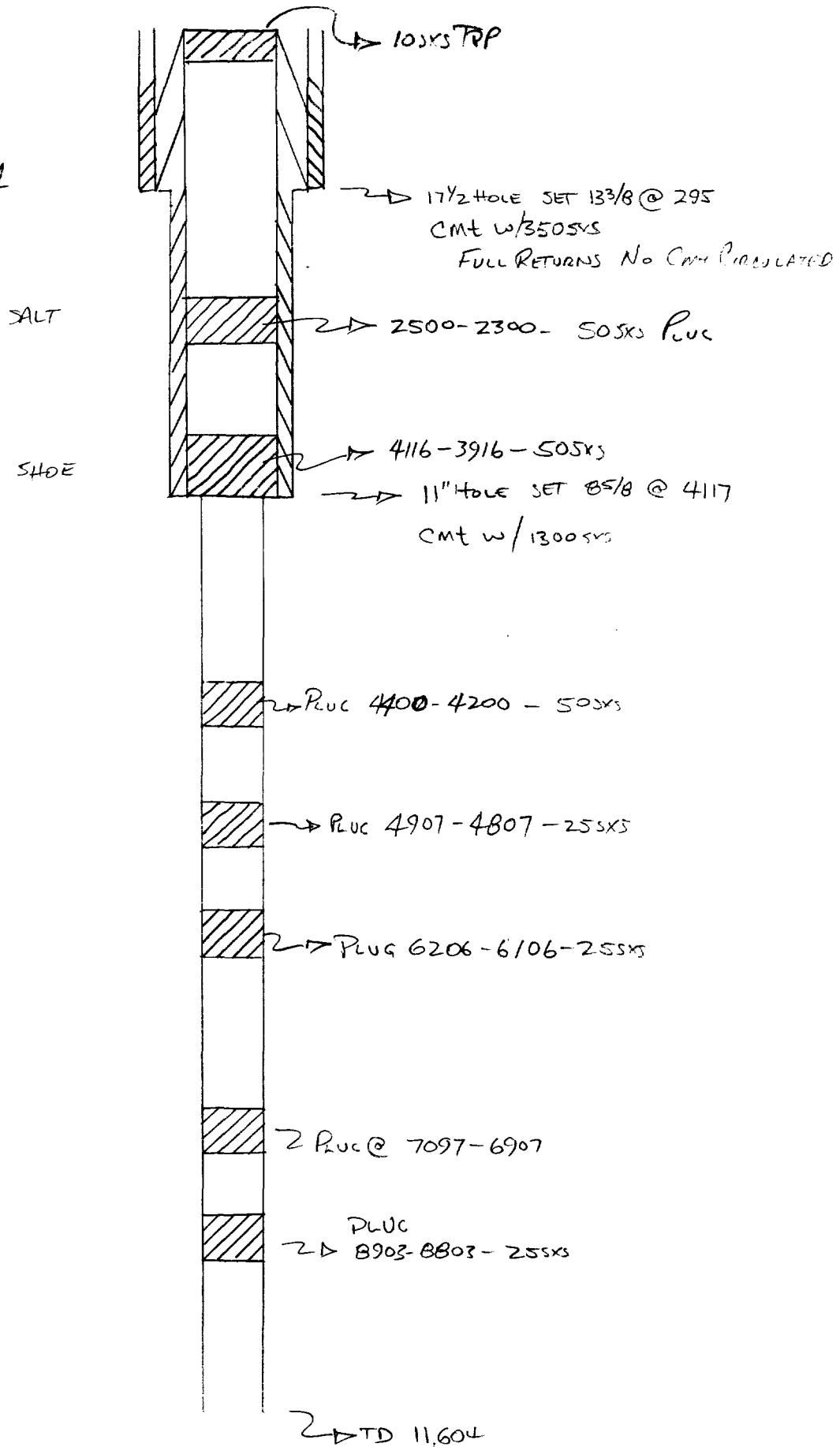
OPERATOR WELL NAME LEGAL & WELL STATUS PERFORATED HOLE SIZE CASING - SET @ — CEMENT — TOP
