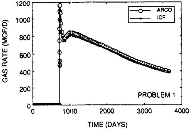
Fig. 7—Gas production rate for Well 3.
