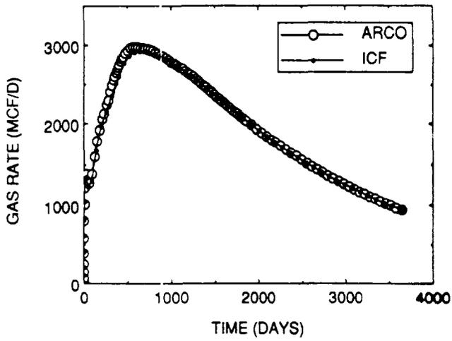
Fig. 11—Total gas production rate vs. time.
