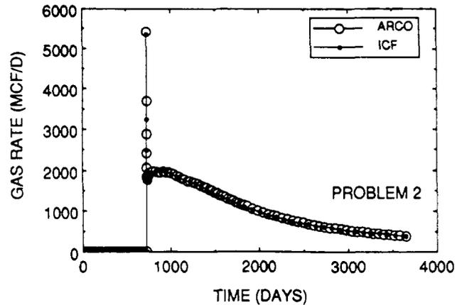
Fig. 12—Gas production rate for Well 3.
