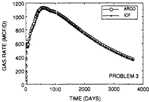
Fig. 17—Gas production rate for Well 3.
