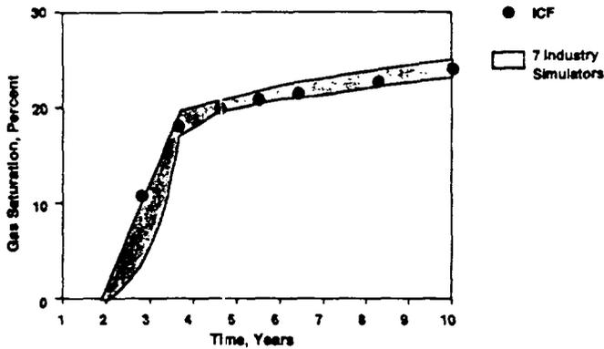
Fig. 21—Gas saturation vs. time for producing Well Cell 10.10.3.
