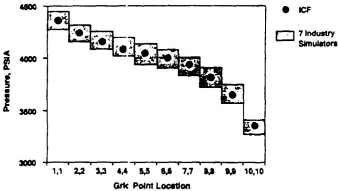
Fig. 23—Pressure vs. grid-point location, time = 8 years, top layer.
