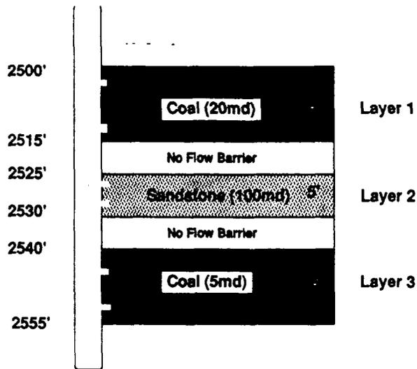
Fig. 2—Well completion schematic for Problem 1.
