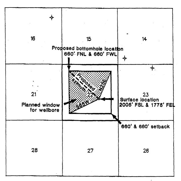
Kickoff Point, Casing Point, Deviation, Azimuth, Bottomhole Location subject to change after logging vertical pilot hole
