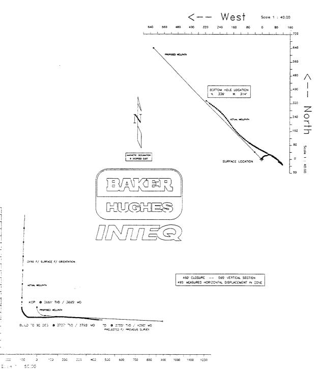
Vertical Section on 315.82 azimuth with reference 0.00 N, 0.00 E from structure
