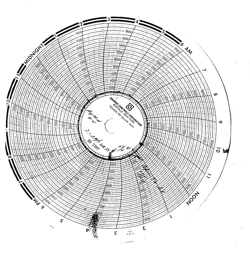
LITTLE SQUAW #1 July 11, 1985 12/64 put on line, came down to line pressure. July 12, 1985 Two (2) hours on line pressure, changed chart. July 13, 1985 Going through separator, line pressure from 2 p.m. to 3 p.m., may have produced some gas. July 14, 1985 Still through separator, riding line pressure. July 23, 1985 Open to air 12/64 choke. July 25, 1985 Flow to burn pit, 12/64 choke, estimated production 400 MCF. July 26, 1985 12/64 choke, estimated production 336 MCF.
