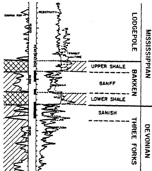
FIG. 2.—Logs from Lloyd H. Smith No. 1-A Weedenman, SE $\frac{1}{4}$  SW $\frac{1}{4}$ , Sec. 29, T. 153 N., R. 94 W., McKenzie County, North Dakota, showing typical productive section. Curve on left is gamma ray. Solid curve on right is resistivity. Dashed curve is interval transit time. Depths (from surface) in feet.
