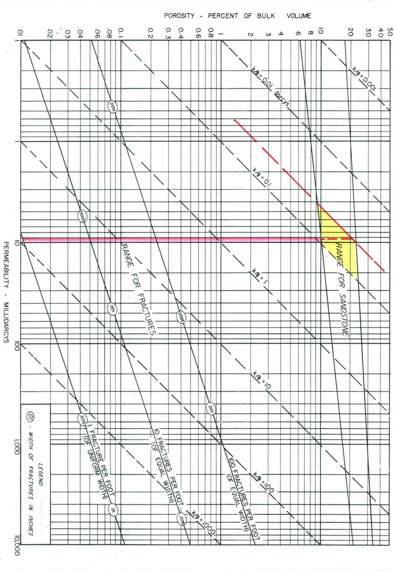
VALUE OF DIFFUSIVITY CONSTANT AS FUNCTION OF  $K/\phi$  VS.  $C\mu$
