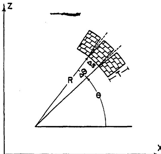
FIG. 3.—Geometry of fracture system used in deriving expressions for fracture porosity and fracture permeability.
